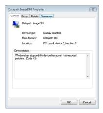
All the cards in your system are driven together to display a single, virtual desktop across multiple screens. Users should be aware that although error code 43 is reported, this is in fact normal operation and there are no faults with the ImageDP4 cards installed in your system.
