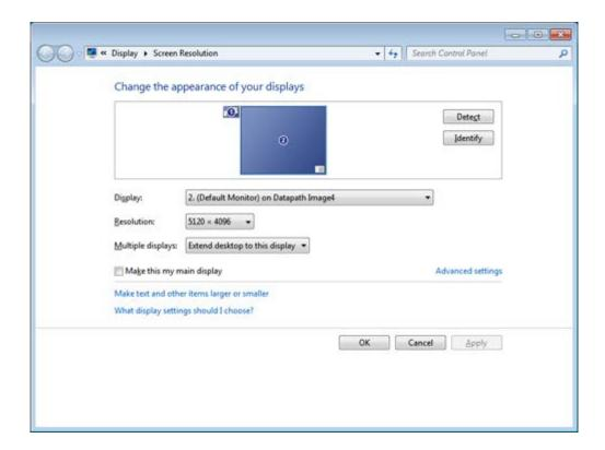
If you have more than one graphics device in your machine, the Display Settings allow you to control which graphics devices are used and what their position on the desktop is. There should be a single monitor icon representing all of the ImageDP4 cards and a monitor icon for each additional graphics device in the system (there is a limit to the number of monitor icons that are displayed).
